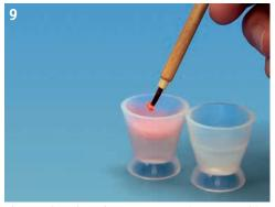
The acrylate has the correct consistency and is A droplet forms. not too liquid.
