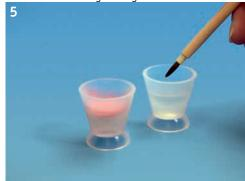
The same amounts of powder and liquid are filled into two mixing cups, separate from each liquid. other.
